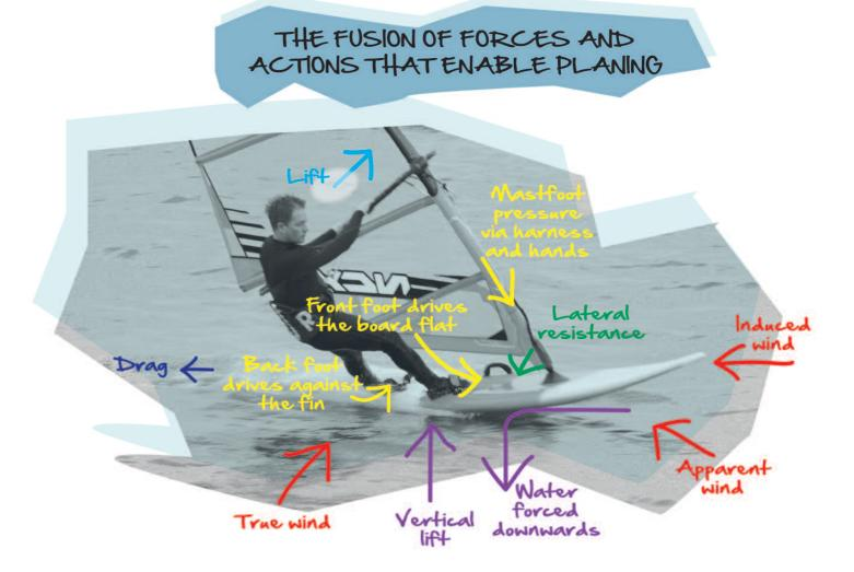
A planing board skims over the surface of the water, having reached a critical speed whereby vertical lift becomes the predominant upwards force
