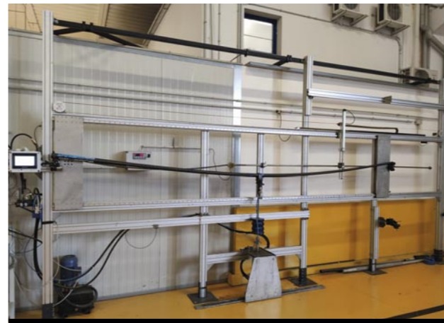
Every mast is deflection tested
