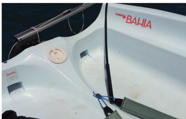
Heaving to: locking-off the tiller leaves both hands free for the helm
