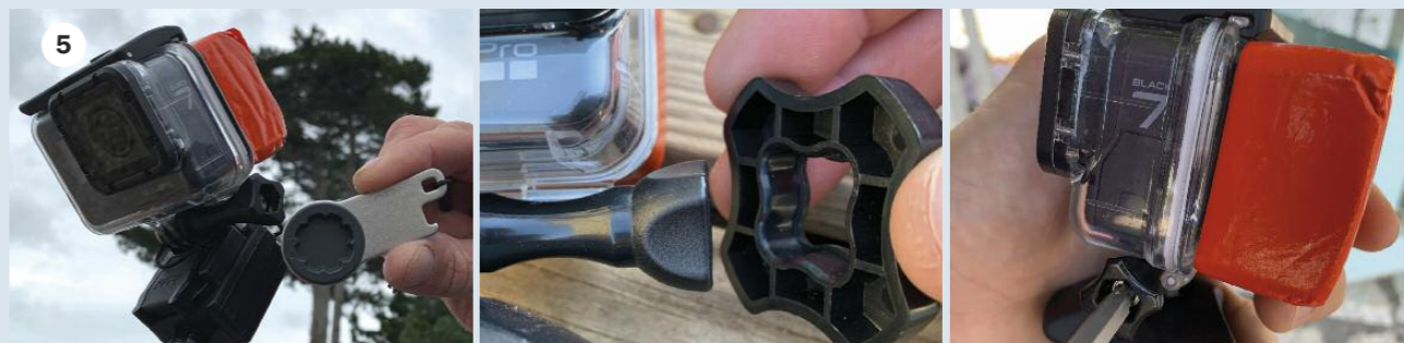
Three ways to tighten your GoPro to any mount (L - R) The Tool by GoPro, The GoBuddy extender or a size 2 Pozi screwdriver
