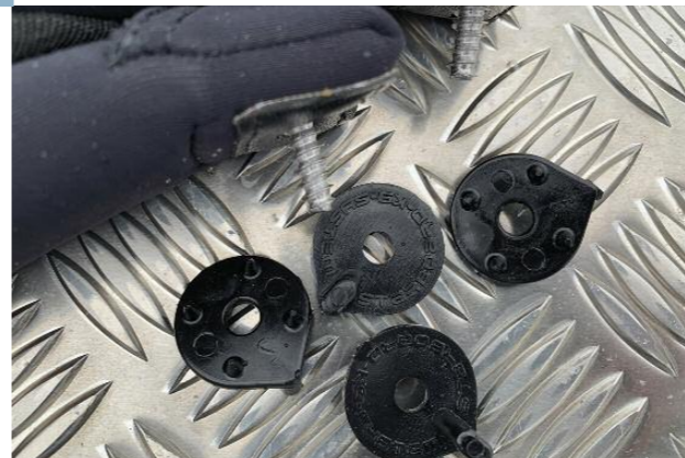
Special long, course-threaded screws and spiky inserts are needed to keep the strap secure and to prevent twist
