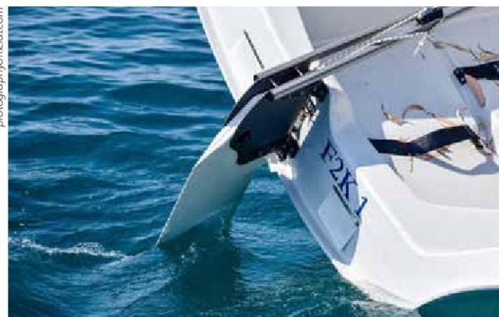
Weather helm makes the flow of water over the rudder blade turbulent which slows the boat down.
