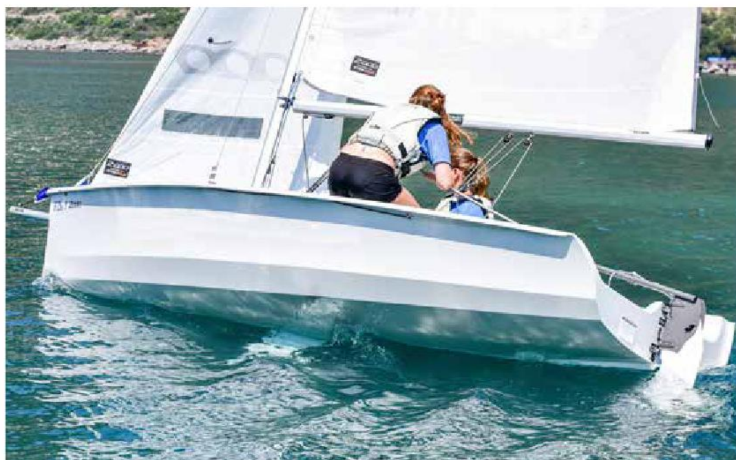
Leeward heel helps with turning towards the wind or can be a nuisance if the boat is kept in a straight line by pulling on the rudder.
